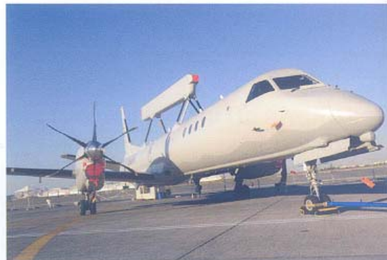
The Pakistan Air Force flew in an Erieye-equipped Saab 2000 for the show
